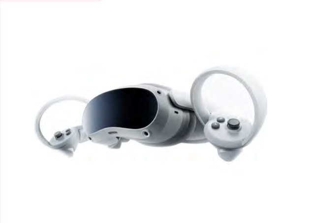
The Pico 4 with its four cameras positioned around the headset's perimeter
