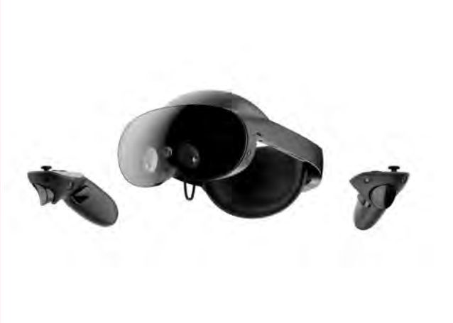
The Quest Pro and its two front-facing passthrough cameras, plus three cameras dedicated solely to inside-out tracking (one on the front and one on each side).
